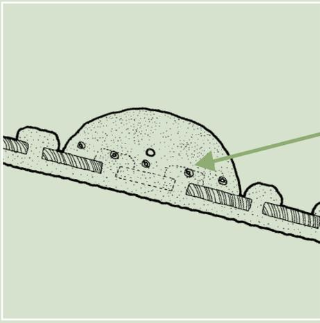
The Plaster of Paris mix is laid over the void left by the removal of the failed lath
