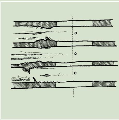
Defective laths are cut off close to the centre line of the timbers behind
