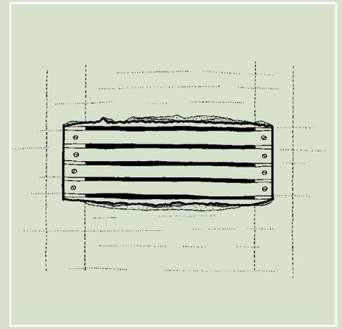
Laths should be replaced with matching sections of timber. The gap between each lath should not exceed the depth of individual laths, but should be adequate to allow the plaster to push through as this is how it is held in place.
