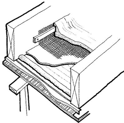
Gauze spreads the load efficiently and reinforces the new plaster layer.
