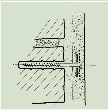
Head of screw is sunken beneath the finished surface of the new plaster
